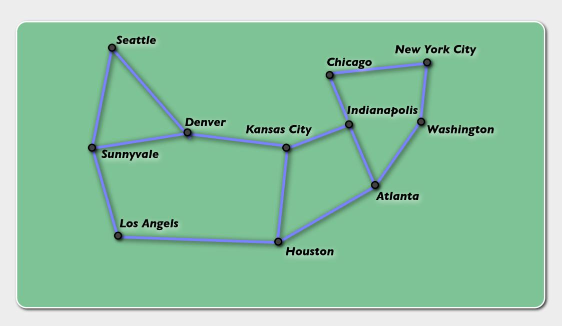
11 nodes with T640 routers, and 14 OC192 circuits.
